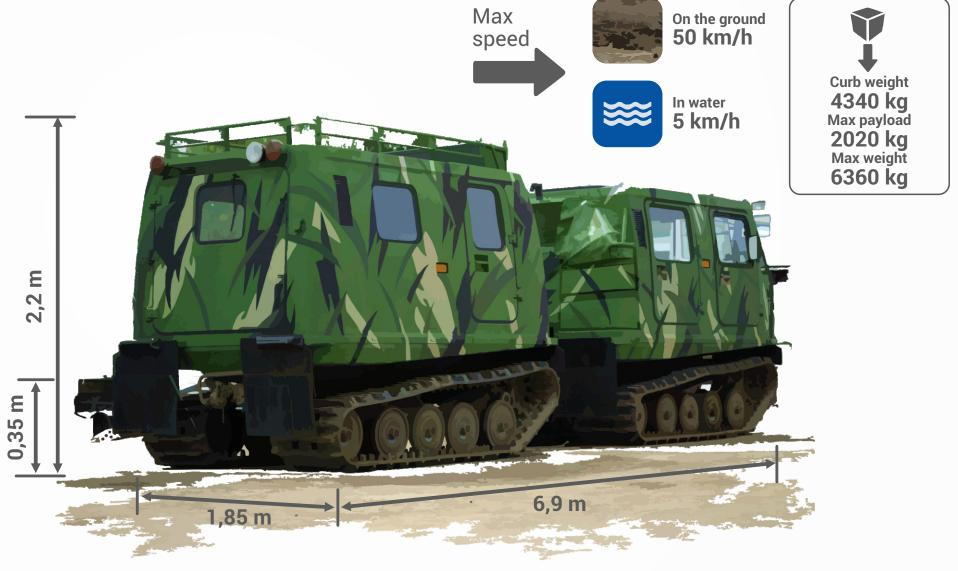
BV-206 is two-section tracked all-terrain vehicle, designed by articulated scheme. Connection of rover sections allows their relative movement in three planes - horizontal, vertical and rotation around the longitudinal axis.
