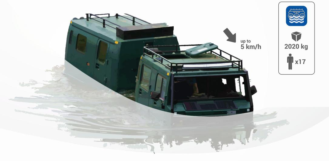
BV-206 is one of the fewest vehicle which is able to swim and move on soft ground at full load. For most of other all-terrain vehicles load limit afloat is 50%. It creates additional expenses while operating all-terrain vehicle.
