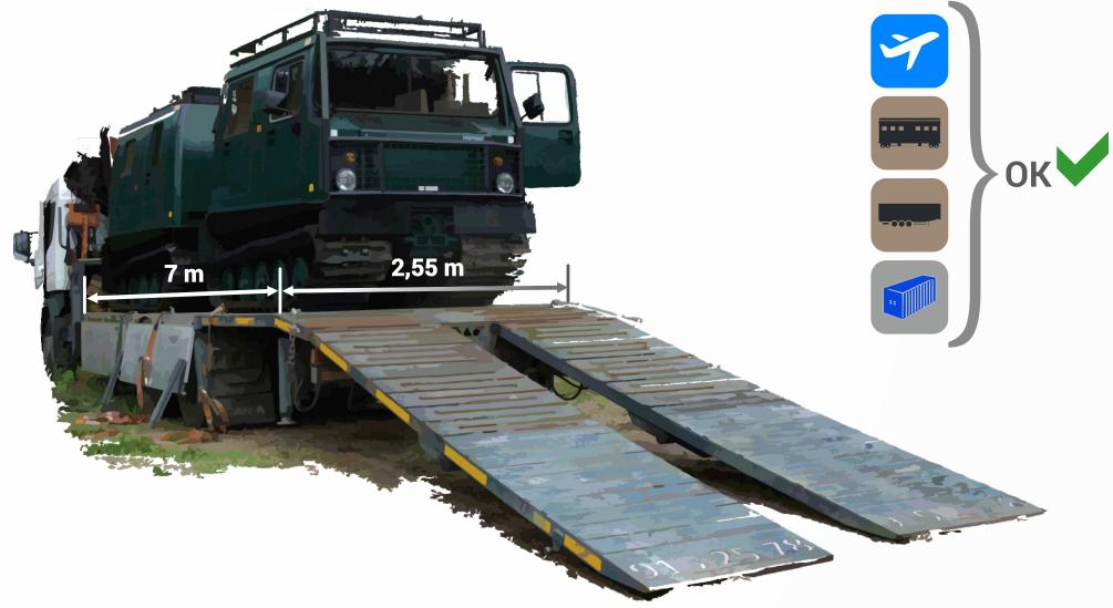
Dimensions and weight allow the vehicle not only to move freely in forests but also to be transported by a "standard" transport – BV-206 can be easily placed in a regular trailer or 40-foot high-cube container. Savings during transportation of the vehicle is up to 30-40%.
